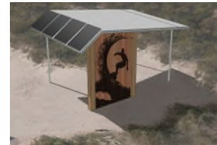
Shelter structure Durable shelter structure with solar panels and battery storage integrated into roof. Site character or unique features represented through materials and sculptural elements, including Aboriginal cultural content.
